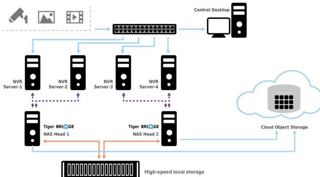
Tiger Bridge allows traditional network video servers to write video feeds to a local drive (or SAN) before being replicated to the object storage. When this object storage is off-premises (in the cloud), this buffer ensures that all video evidence is recorded prior to being encrypted and transferred to the cloud. Since Tiger Bridge runs directly in the server's memory, https encryption takes place before any critical data goes on the network, ensuring that data is secure. Once in
